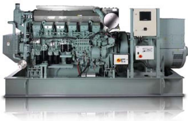
Individual cylinders heads, large inspection and maintenance covers on both sides of the engine enable easy access to all main parts. Turbochargers, injection pumps and water pumps have a fully integrated lubricating oil system with changeover lubricating oil filters. Compact in design, the generator set occupies less space in the engine room and its good accessibility makes service and maintenance easy.
